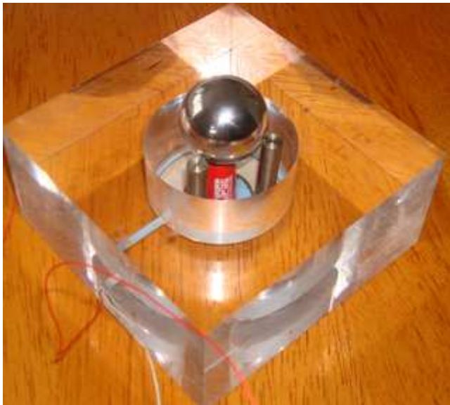
Fig. 7 Fabricated Prototype of the proposed 3D USM using a single piezo-ceramic flexural vibrating ring transducer
