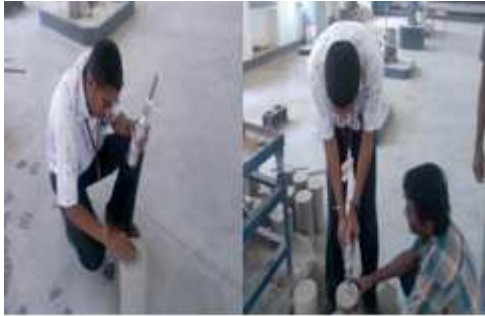
Fig. 2 Non – Destructive test (Rebound Hammer) on cylinder
