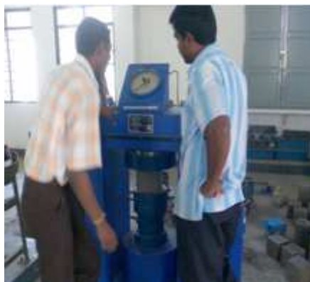
Fig. 4 Compression tests for cubes
