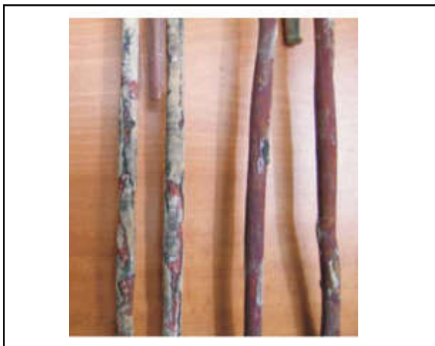
Fig. 4 Copper coil corrosion
