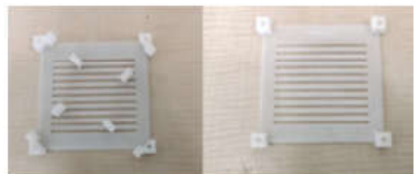
Fig.6 Front and back plate of the CubeSat
