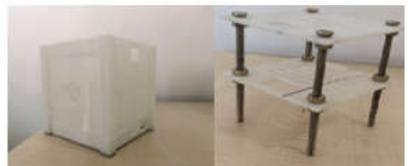
Fig. 5 Main body and frame structure of the cubesat
