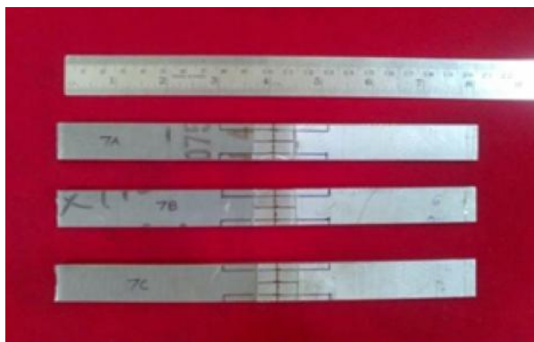
Fig.5 Preparation of tensile specimen from Friction stir welded plate
