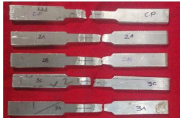
Fig 8 Tensile specimen after fracture
