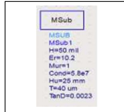
Fig.3 Substrate parameters of RTDuroid 6010
