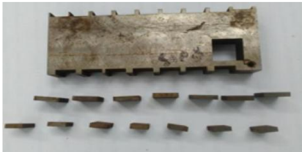
Fig. 2 Machined work piece with cut pieces
