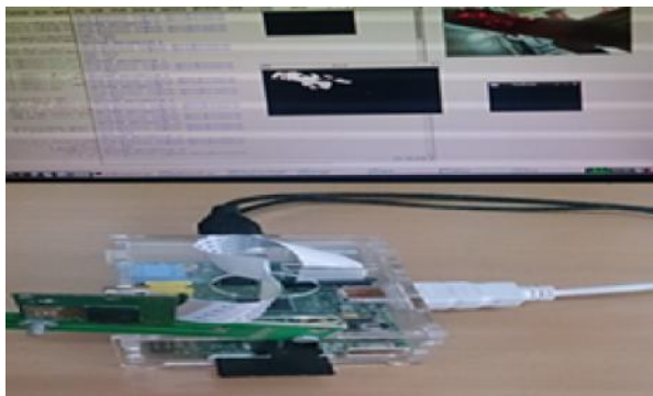
Fig.9 Raspberry Pi interfaced with Raspbian camera with the monitor window
